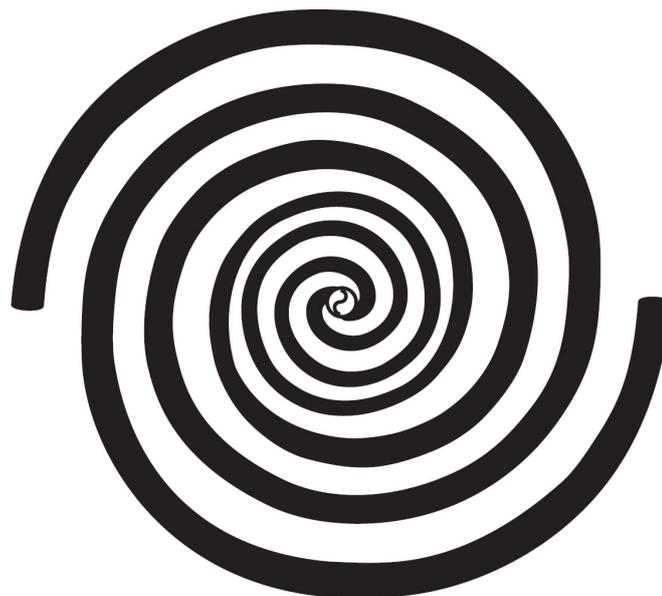
**Figure 1.10:** Self-complementary planar spiral antenna structure [31].
