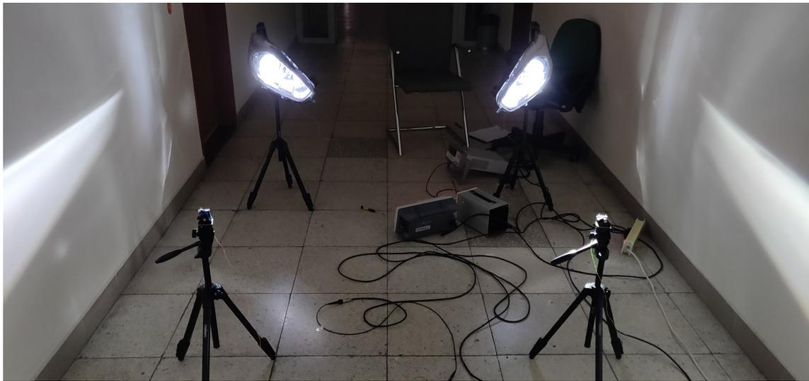
**Figure 2.21:** Indoor laboratory measurement setup, for 2x2 D-SD vs. 2x2 C-SD comparison with deactivated common-mode noise source.
